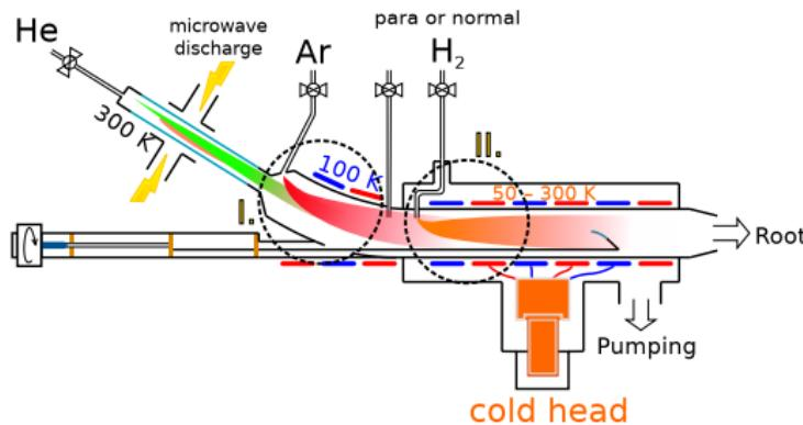
Flowing afterglow – production of  $H_3^+$ -e<sup>-</sup> plasma step by step
